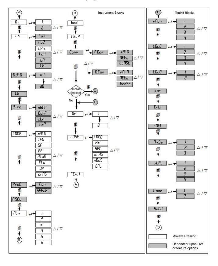
Press to scroll through each list header (the name of the function block) in turn
