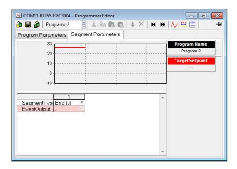
Up to 10 stored programs can be configured. By default, a stored program will consist of just an End segment as shown above.
