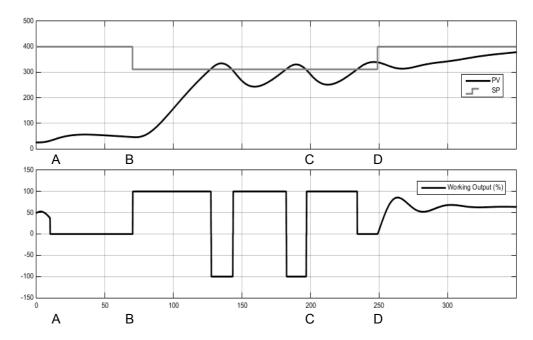
The third shows an example of Heat/Cool Autotune from above with output rate limiting.
