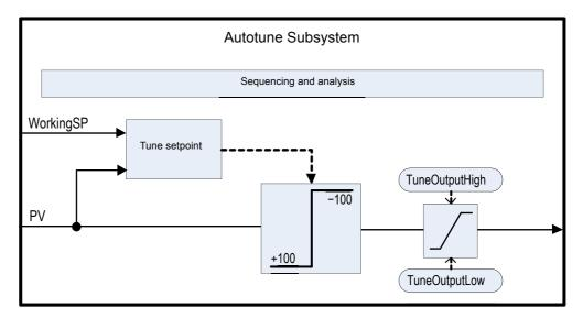
The function block contains sophisticated autotuning algorithms that can tune the controller to the process. They work by performing experiments on the plant, by inducing perturbations, and observing and analysing the response. The autotuning sequence is described in detail below.
