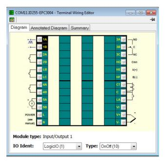
From this view click on a set of terminals. In the 'IO Ident' drop down select an IO type. The diagram of the type of IO will be shown against the chosen terminal set.
