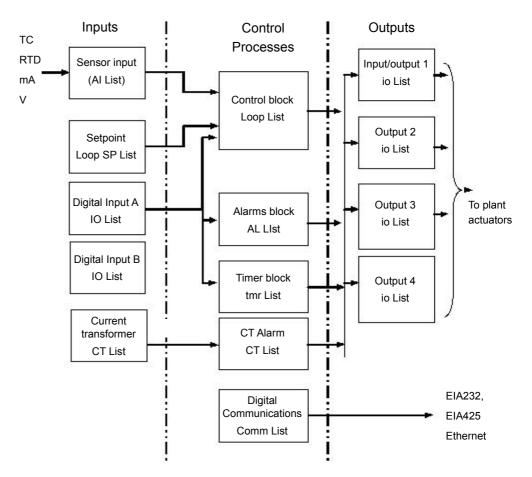
The Temperature (or Process Value, PV) is measured by the sensor and compared with a Setpoint (SP) set by the user.
