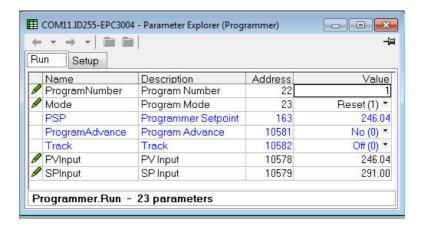
To run a stored program make sure that the controller is in Operator mode. Select the stored program number of the program to run and select Run(2) from the Mode parameter drop down enumeration. The program may also be put into Hold or Reset from the mode Parameter.
