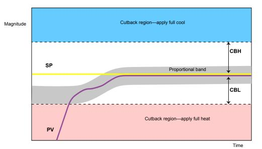
**Note:** Because cutback is a type of non-linear controller, a set of CBH and CBL values that are tuned for one particular operating point may not be satisfactory for another operating point. It is always advisable therefore not to try to tune the cutback values *too* tightly, or otherwise to use gain scheduling to schedule different values of CBH and CBL at different operating points. All the PID tuning parameters can be gain scheduled.
