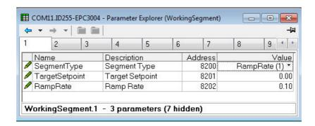
The Working Segment provides the user read/write access to the segment parameters of the currently running program (which can be the main program or a subroutine resulting from a call segment).
