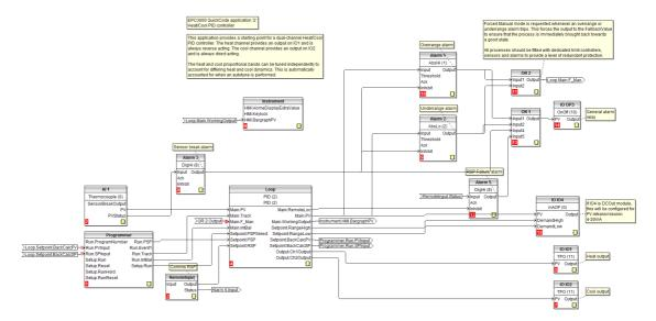
This is the same as the heat only controller but with the addition of IO2 connected to the cool output.
