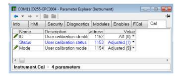
It may be found useful to open the Al1 browser list when carrying out the calibration since the PV can be read directly during the calibration procedure. This also allows the input measurement settling to be viewed during the calibration process.
