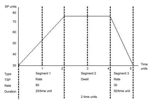
The example above shows a simple three segment program in which the programmer setpoint (PSP) increases at a controlled rate of 25/time unit to a value of 80. It then dwells at that setpoint for 2 time units before decreasing to 30 at a controlled rate of 50/time unit.
