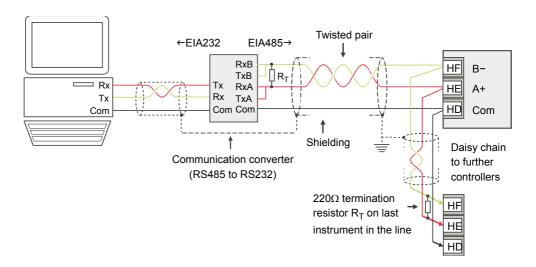
**Note:** The device physical interface can only support up to 31 devices for each segment. More than 31 devices will require additional buffering. For more details see the Communications Manual HA026230 which can be downloaded from www.eurotherm.co.uk.
