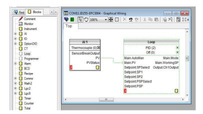
A list of function blocks is shown in the left hand side. Blocks are dragged and dropped from the list into the Graphical Wiring section on the right.
