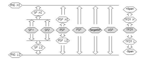
The Span is taken to be the value given by (RangeHigh – RangeLow).
