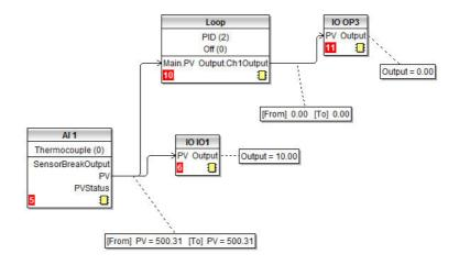
The diagram shows a simple loop where the control output is connected to Output 3 and the PV is wired to Analogue Output 1 configured for 0 - 10V.
