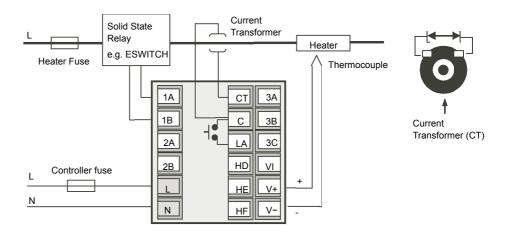
**Note:** A burden resistor value  $10\Omega$  is mounted inside the controller.
