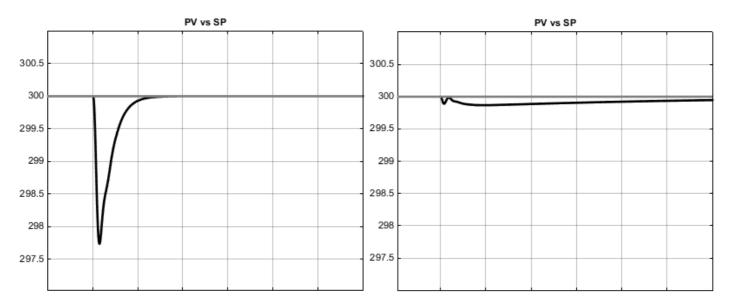
Here, it can be seen that enabling power feedforward has greatly reduced the magnitude of the process disturbance. However, the smaller disturbance persists for a longer period of time.
