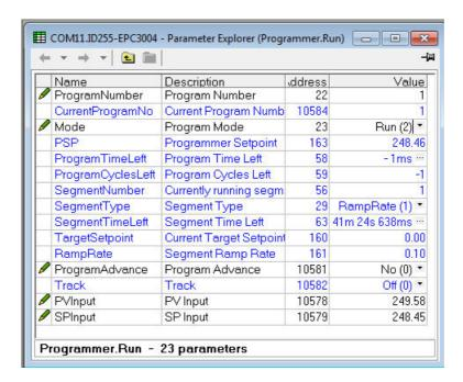
When one of the stored programs (Program 1 to 10) is run, the stored program parameters are copied into the working program. The Working Program and Working Segment parameters are then made available to the user for monitoring and/or editing.
