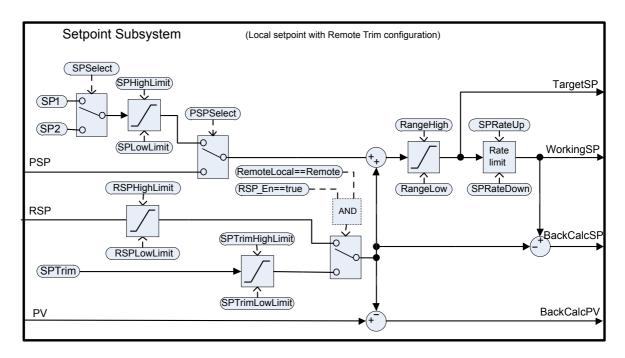
The setpoint subsystem resolves and generates the working setpoint for the control algorithms. The working setpoint can ultimately come from several different sources, programmer, local or remote, have local or remote trims applied, and be limited and rate limited.
