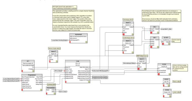
This is the same as a heat only controller except that IO1 and IO2 are configured for valve raise and valve lower respectively.
