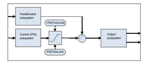
A symmetrical trim limit is provided around the PID component such that the influence of the feedback trim can be restricted.
